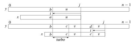
Algorithm Turbo-BM uses the lengths mem = |u| of the previous suffix match u and  $\ell = |v|$  of the current suffix match v to compute  $\max\{good\text{-suff}[i], |u| - |v|\}$ .
