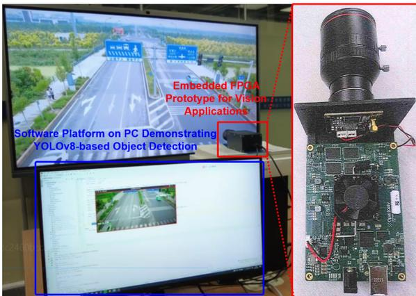
Fig. 9. Demonstration of a camera-equipped FPGA hardware prototype and PC-based software platform for YOLOv8 object detection
