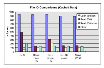
File opening took roughly the same time for all methods. File closing consistently took a little longer for C IO. All reading was slow for C++ stream IO, whereas the caching system of C IO caused first reads to be slow, but subsequent reads to be fast. C low level IO, C++ file class, and native OS all reads took basically the same
