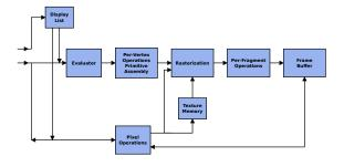
An illustration of the graphics pipeline process
