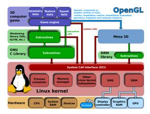
Video games outsource real-time rendering calculations to the GPU over OpenGL. The rendered results are not sent back, and are instead stored in a framebuffer whose content is sent to the display controller.
