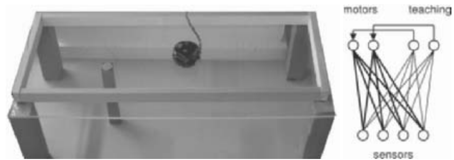
Figure 6.52 Left: A Khepera robot gains fitness points by finding and staying over a movable target area located on the floor. The walls are covered with white (image) or black paper that changes every generation. The robot has a ground sensor that can detect the target area when it passes over it. Right: Self-teaching network. The output values of two teaching neurons are used as teaching values of two motor neurons. The weights that connect the sensory neurons to the teaching neurons do not vary during the robots' lifetime while the weights that connect the sensory neurons to the motor neurons are modified by backpropagation of error.
