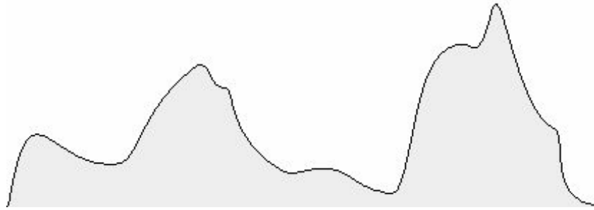
Figure 5.14: Graphical representation of a fitness landscape illustrating the peaks towards which the most fit solutions of a GA migrate and the valleys in which the least fit lie. Note that there can be peaks of varying heights.
