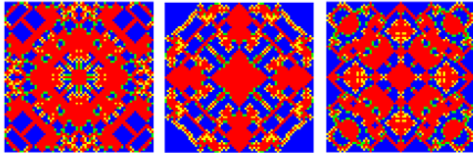
Figure 5.12: Employing a von Neumann neighborhood, these are three images in the time-evolution of the spatial prisoner's dilemma with a value of b = 1.4 and an initial sole defector set in a sea of cooperators. Periodic boundary conditions are used. The color code is: blue = cooperators, green = new cooperators, red = defectors, yellow = new defectors. Implementation by Christoph Hauert.
