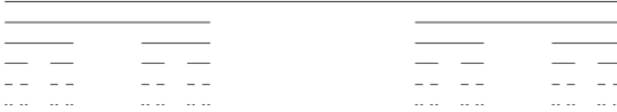
Figure 1.13: The construction of the Cantor set whereby the middle third of each remaining line segment is removed. Image courtesy G.W. Flake, The Computational Beauty of Nature .
