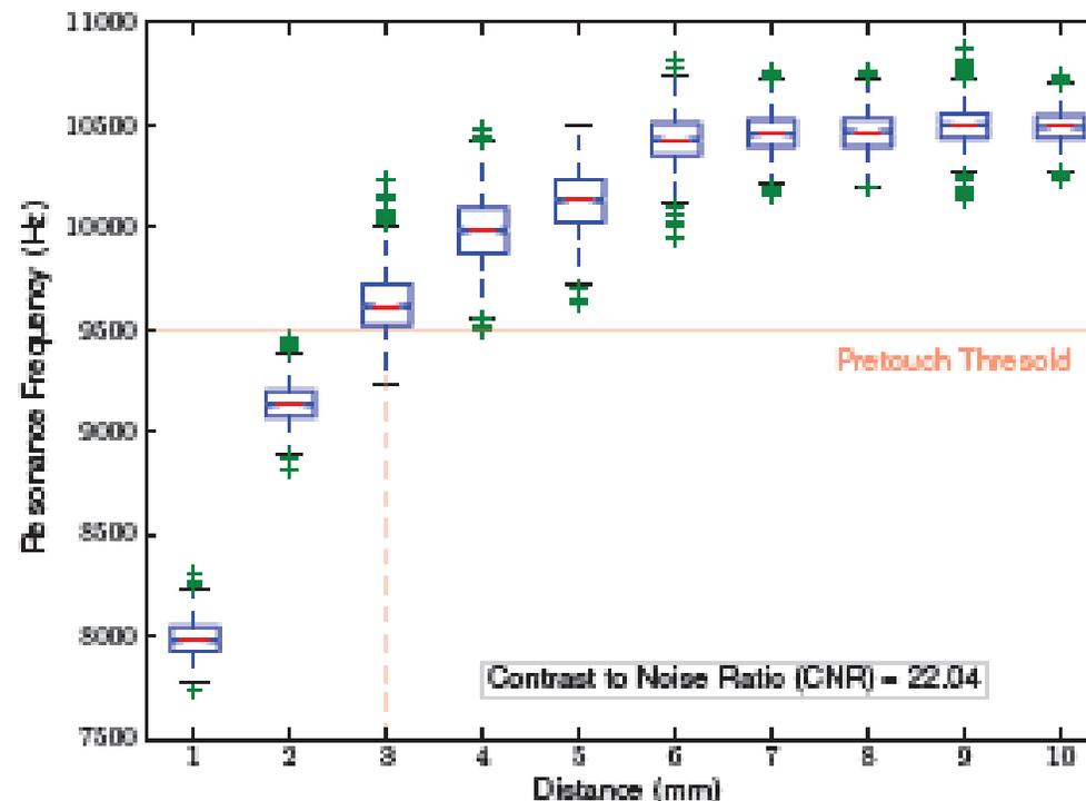
The box and whisker plot of 1000 estimated resonance frequencies at 1-10 mm.
