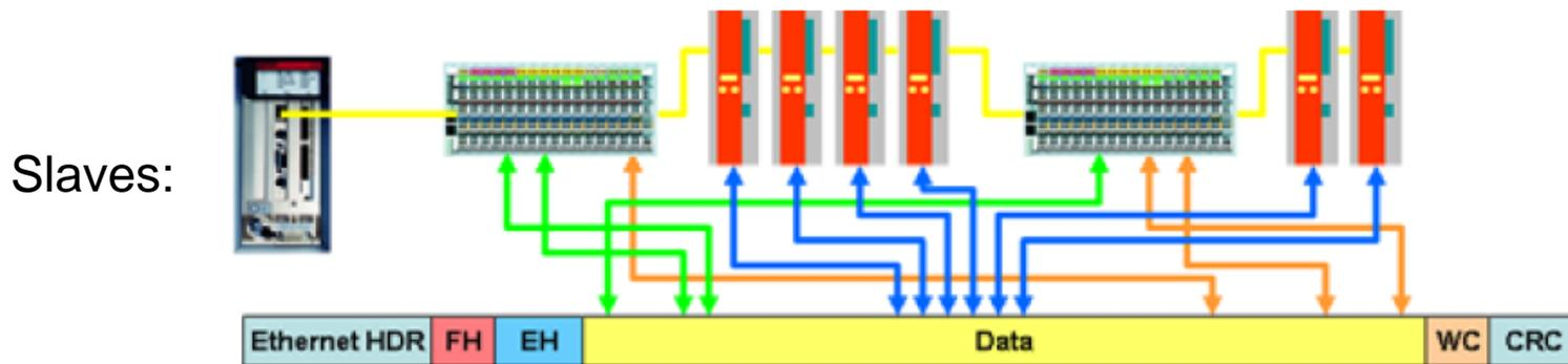
*Figure 4: Devices map data directly in frame*
