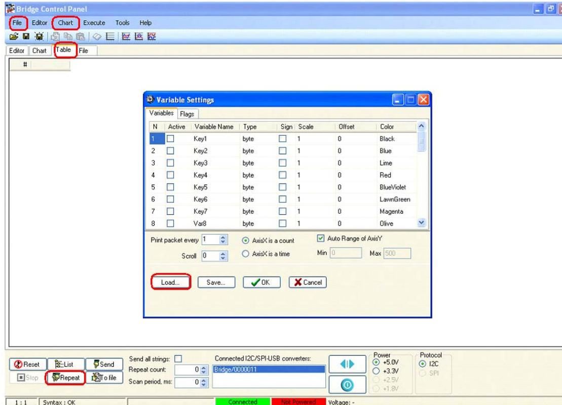
2. Load the *demo.ini* file by clicking the **Load** button, as shown in Figure 3-7. The *demo.ini* file initializes light and temperature variables and is available in the CY3240-I2USB kit CD or at the following location: <Installed\_directory>:\Cypress\CY3240-I2USB.
