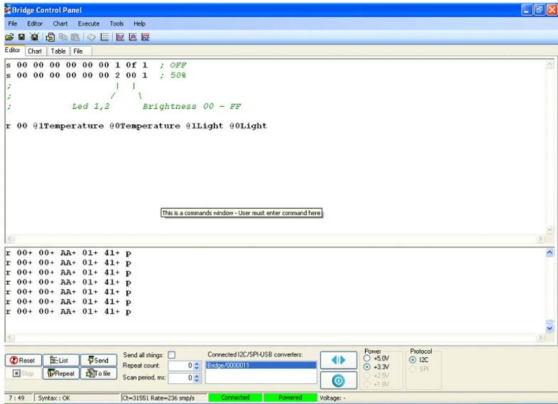
5. Click in the last line, which reads temperature and light data from the device and then click the **Repeat** button. On clicking **Repeat**, the command that is sent last is repeated until **Stop** is clicked. This makes data collection easier. The data received from slave can be viewed either graphically or in a tabular form.
