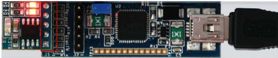
2. Select **+5V** as power supply to the board from Bridge Control Panel. The LED (red) on the bridge board lights up, as shown.
