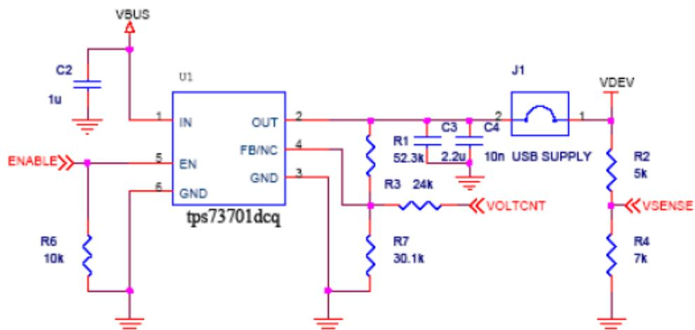
Figure A-2. USB Connection with Voltage Suppressor Schematic
