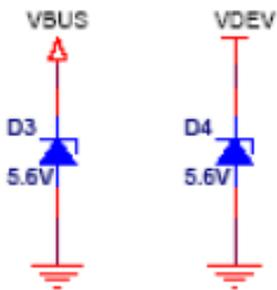
Figure A-4. Voltage Regulator Schematic
