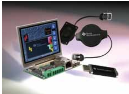
▲ Stellaris RDK-IDM-SBC single-board computer intelligent display reference design kit
