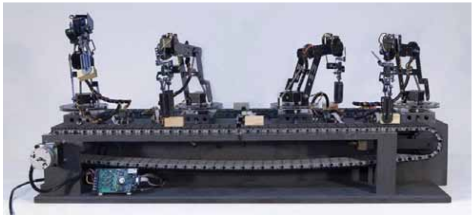
▲ Stellaris Ethernet + CAN factory automation demonstration
