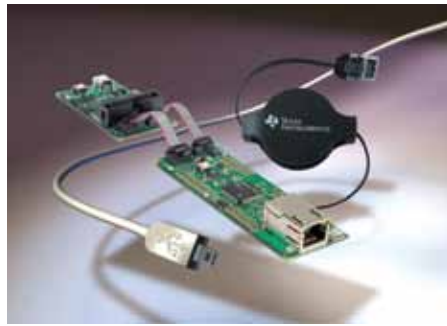
▲ Stellaris EK-LM3S9B92 quickstart Ethernet + USB evaluation kit
