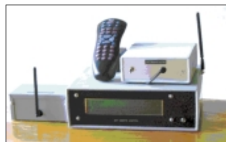
Photo 1: This photo shows the various parts of the system. The mini-box to the left houses the 433-MHz receiver. The case with the large LCD is the MP3 remote control unit. Sitting above it are the RCA remote control and the FM broadcaster module. In normal use, only the FM broadcaster and receiver are located with the host computer, the remote controller is placed wherever you want to listen to the MP3 music.
