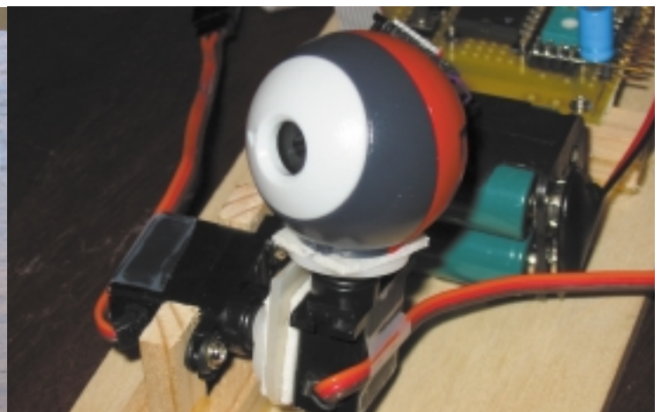
Photo 6a: Four AA NiCd or NiMH batteries power the circuit board used for the pan-tilt head. b— These servos have a quick transit time. It takes only 0.09 s to rotate the control surface through 60°! This fast response time keeps the servos from being the limiting factor in the system's reaction time.
