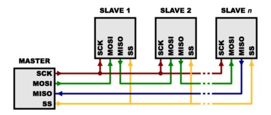
Note that, for this layout, data overflows from one slave to the next, so to send data to any *one* slave, you'll need to transmit enough data to reach *all* of them. Also, keep in mind that the *first* piece of data you transmit will end up in the *last* slave.
