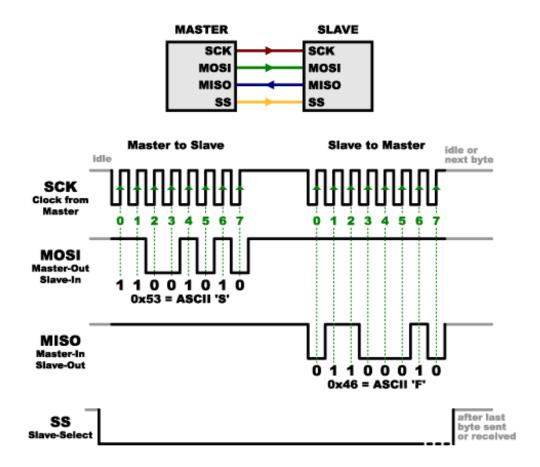
The SS line is normally held high, which disconnects the slave from the SPI bus. (This type of logic is known as "active low," and you'll often see used it for enable and reset lines.) Just before data is sent to the slave, the line is brought low, which activates the slave. When you're done using the slave, the line is made high again. In a <u>shift register</u>, this corresponds to the "latch" input, which transfers the received data to the output lines.
