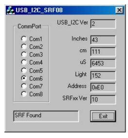
The connector on the USB-I2C module may be soldered directly to the SRF08 as shown, or you can use a cable if preferred. The USB-I2C module can easily supply the 25mA peak of the SRF08. The software automatically searches for the SRF08 and displays its I2C address, along with revision number, range and light sensor reading. Download <a href="mailto:usb\_i2c\_srf08.exe">usb\_i2c\_srf08.exe</a> and the <a href="mailto:C source code">C source code</a> here.
