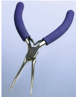
Figure 1-2. Longer-nosed pliers: these are useful for reaching into tiny spaces.
