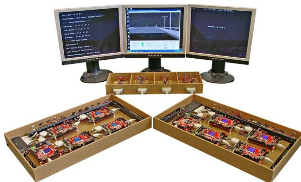
Figure 107: An example of a simulation framework used to perform initial tests on an automotive control system. Photo by Peter Vidler.
