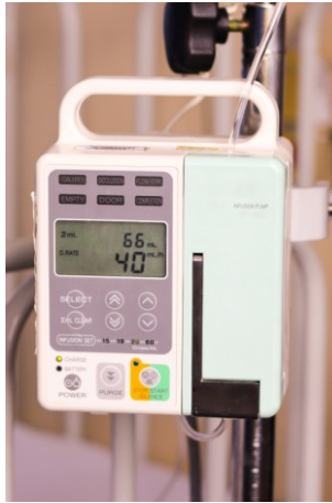
Figure 105: An example of a medical infusion pump (an external pump). Licensed from: Dreamstime.com. Photographer: Abubjism.
