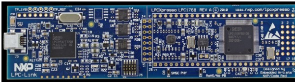
Figure 122: The LPC1769 board. Photo from NXP.
