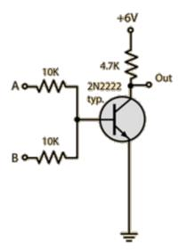
transistors for the construction of logic gates depends upon their utility as fast switches. When the base-emitter diode is turned on enough to be driven into saturation, the collector voltage with respect to the emitter may be near zero and can be used to construct gates for the TTL logic family. In this
