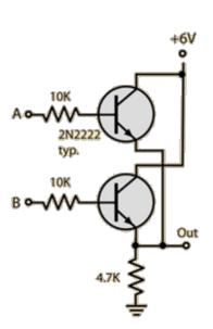
The use of transistors for the construction of logic gates depends upon their utility as fast switches. When the base-emitter diode is turned on enough to be driven into saturation, the collector voltage with respect to the emitter may be near zero and can be used to construct gates for the TTL logic family. For the OR logic, the transistors
