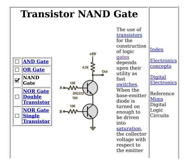
may be near zero and can be used to construct gates for the TTL logic family. For the NAND logic, the transistors are in series, but the output is above them. The output is high unless both A and B inputs are high, in which case the output is taken down close to ground potential.
