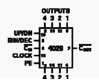
the counter to operate in binary mode, while a logic 0 switches it to decimal (sometimes called *decade*) mode. If multiple 4029s are cascaded for a larger count, all **up/dn** pins are connected together and driven from a common signal, as are all **bin/dec** lines.
