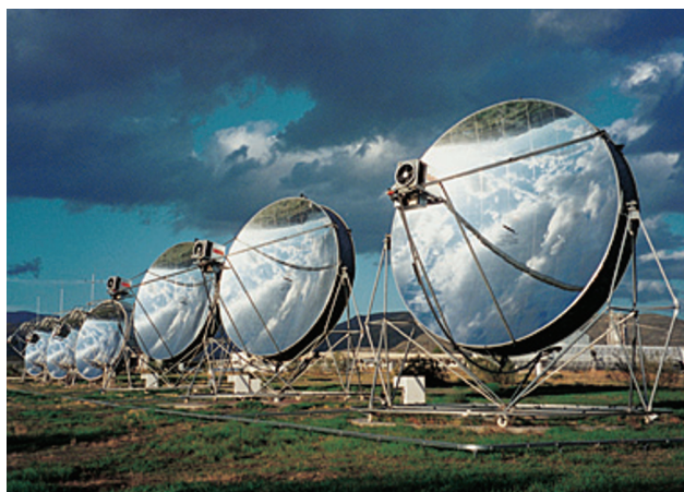
Figure 4. Parabolic sun collectors (source: DLR).
