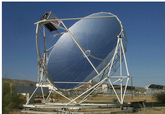
Figure 5. EuroDish system (source: Wikimedia Commons).
