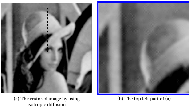
FIGURE 3.15 Restored images obtained by using isotropic diffusion: (a) the restored image by using isotropic diffusion, and (b) the top left part of (a).
