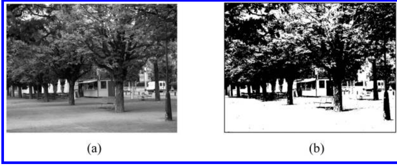
FIGURE 4.3 optimal thresholding: (a) original image, and (b) optimal thresholding segmentation (optimal threshold = 115).
