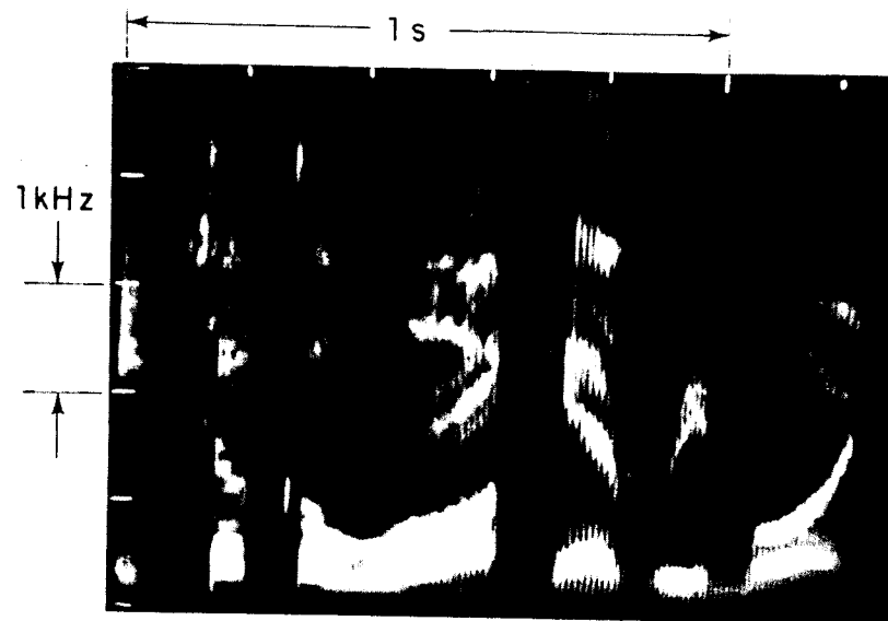
Fig. 6.39 An example of a spectrogram produced using the short-time spectrum and a computer graphics system. (After Oppenheim [14].)
