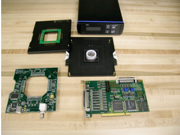
Fig 2. Data acquisition system including (from top left to bottom right) amplifier, MEA temperature controller, MEA, MEA amplifier base, 64 channel stimulator, and PCI data acquisition card from MultiChannel Systems.
