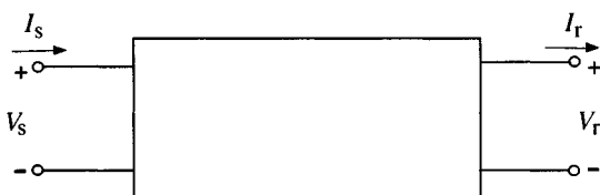
Fig. 8.9. Reference directions for current and voltage variables for ABCD parameters.
