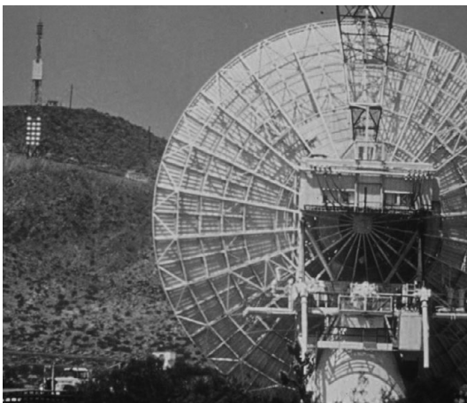
Figure 6.24 Wireless power transmission experiment at Venus JPL cite. ©1984 IEEE. Reprinted with permission from [126]
