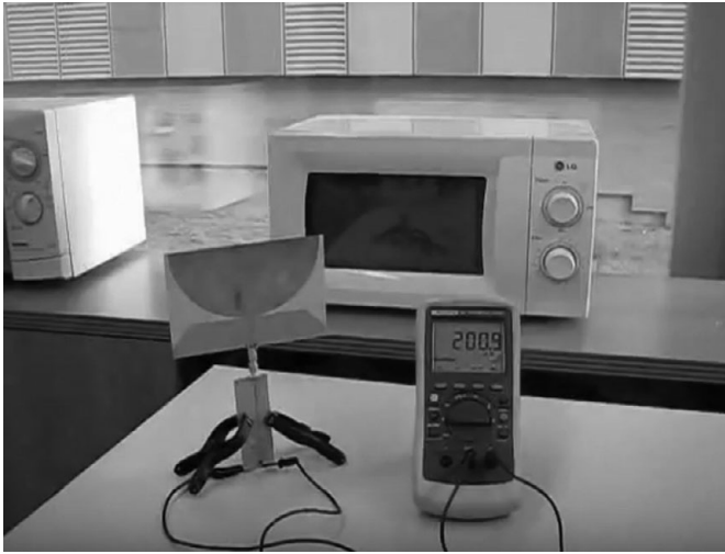
Figure 7.1 Harvesting the leaked signal from a commercial kitchen microwave.
