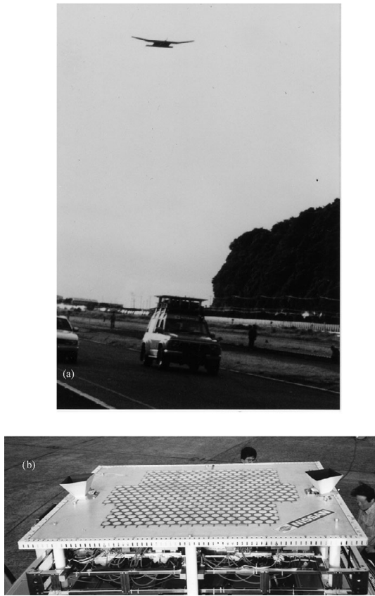
Figure 6.25 Airplane powered by a microwave beam from a phased array antenna: (a) flight experiment, and (b) antenna array [178]. Photos courtesy of Prof. Naoki Shinohara, Kyoto University
