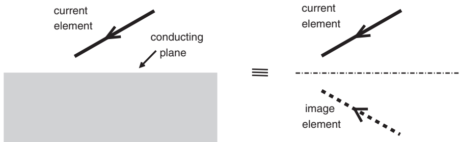
Fig. 8.11 Current element over a conducting plane and equivalent system that uses an image element.
