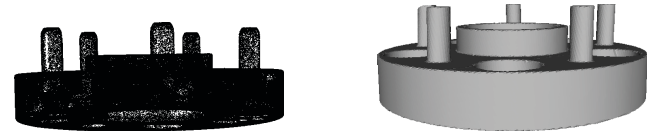
Fig. 9. A more complex CAD part recovered by our approach. Left: The input point-cloud. Right: The meshed recovered expression.
