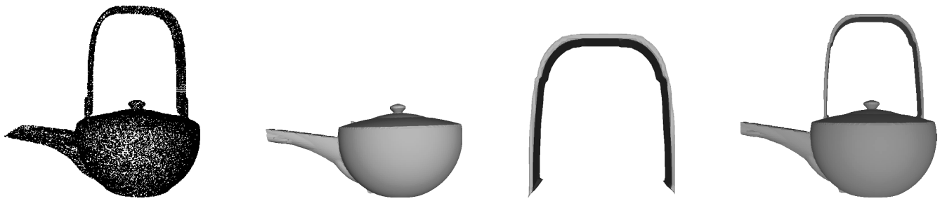
Fig. 10. User-assisted reverse modeling. Left: The original point-cloud. Middle: Intermediate object with the handle missing. Right: Final object with the handle fitted and attached to the object with the union operation.
