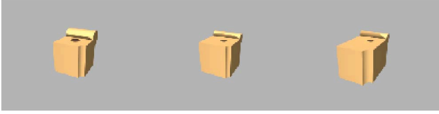
Fig. 4. Illustration of a parameterized template model: a model is built in a constructive way with abstract parameters (corresponding to the position and radius of the cylinders, lengths of the box) that can be tuned to satisfy some modeling criteria. The images from left to right show the model with different parameter values.
