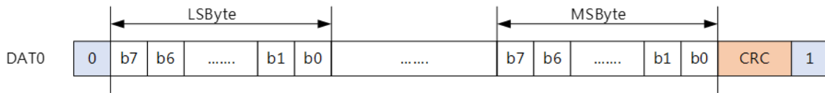
Diagram 21.24: eMMC/SD/SDIO 1-bit data packet format
